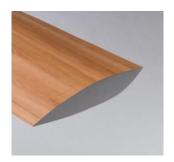
EGGER Laminate MED is a decorative laminate based on curable resins. The laminate is constructed by fusing multiple layers and consists of melamine resin impregnated decor paper and several phenolic resin impregnated core layers. EGGER Laminate MED is suitable for all uses / areas of application as outlined below and in addition meets the requirements of the Marine Equipment Directive with regard to:
